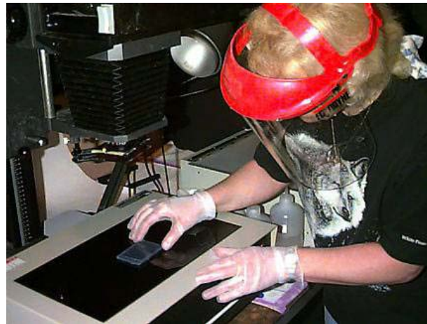
④ Use UV to visualize DNA (UV fluorescence dye was added before loading)
