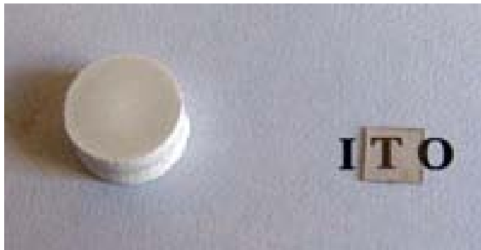
A pellet of Indium Tin Oxide sample (left) and this same material in thin film form (right)
