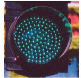
Fig. 1.12. Green traffic signals are one of the ubiquitous applications of GaInN/GaN green LEDs.
