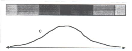
C denote the linear concentration of contaminant. The diff usive discharge Q<sub>d</sub> of contaminant, in grams grossing a se ction as s per unit time, is taken to be given by Fick's law.
