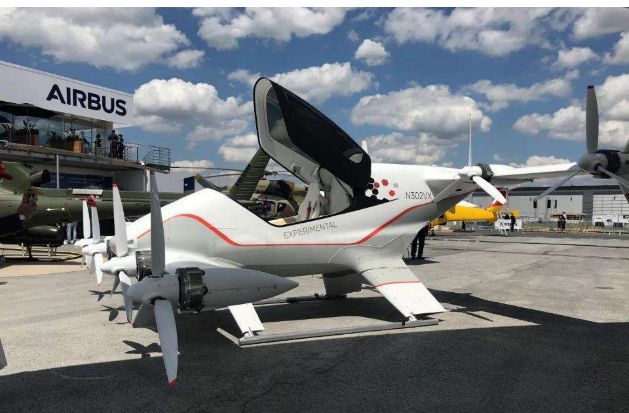
Airbus A 3 Vahana Tiltwing demonstrator (vectored thrust)
