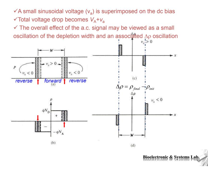
✓ Effectively, it looks like plus and minus charges are being alternately added and subtracted from two planes separated by a width W.
