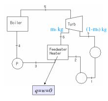
eXtreme Combustion Laboratory • Example of Regeneration cycle Given steam enters turbine at  $p_5 = 4MPa, T_5 = 400^{\circ}C$   $\Rightarrow$  superheat
