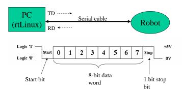
• Why we need start bit in asynchronous communication even when the both sides use the same baud rate?
