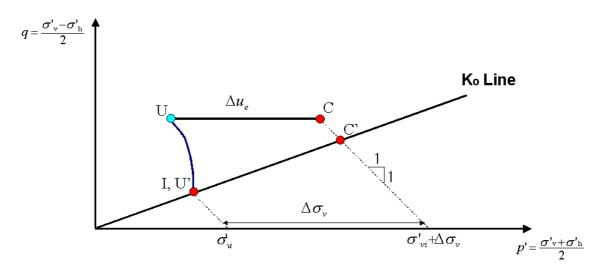
U'C': Consolidation path of oedometer test.
