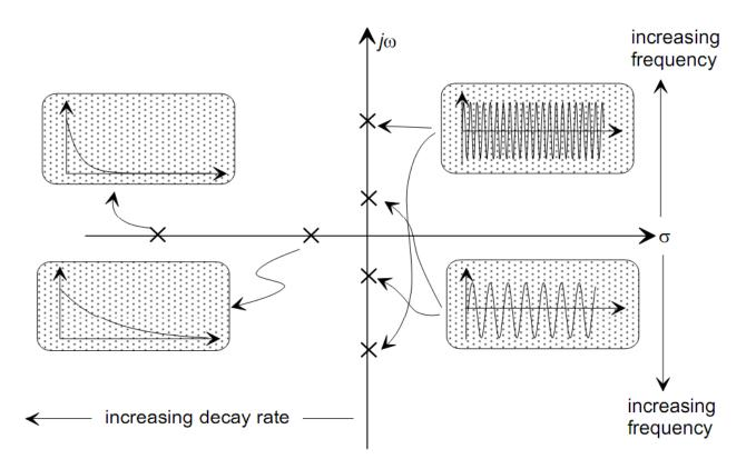
5) the oscillatory frequency and decay rate is determined by the distance of the poles from the origin.
