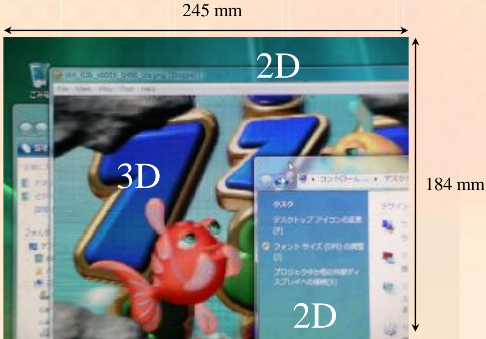
Prototype of 2D/3D switchable display
