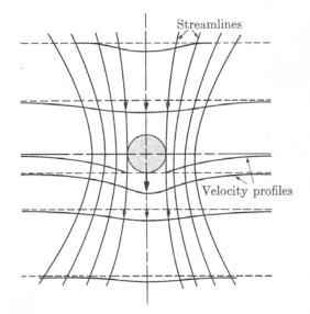
FIG. 8–3. Deformation flow around a falling sphere. (Streamlines and velocity profiles are shown for observer at rest.)
