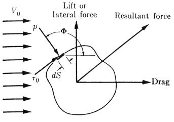
FIG. 8-7. Definition diagram for flow-induced forces.
