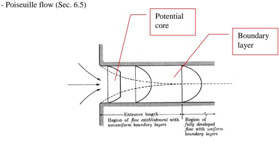
FIG. 8-5. Boundary layers in ducts.
