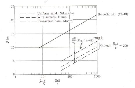
FIG. 12–11. Example of roughness types and definitions of roughness magnitude k.
