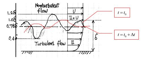
(1)Average position of the turbulent-nonturbulent interface = 0.78  $\delta$
