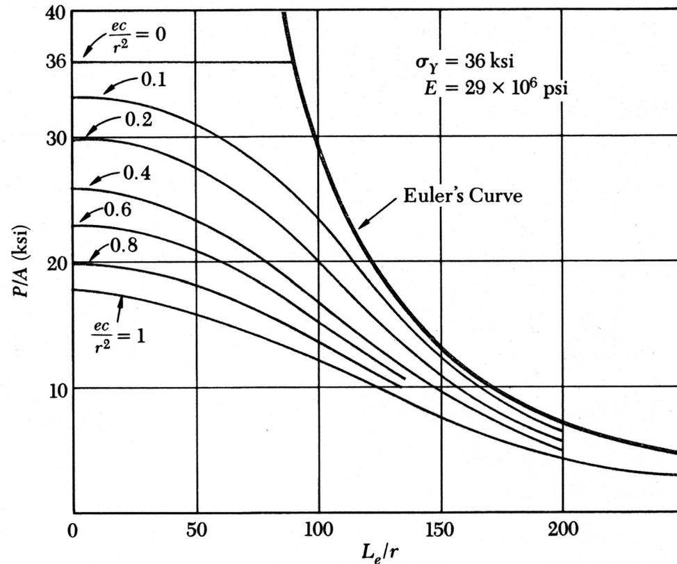
Fig. 11.23 Load per unit area,  $P/A$ , causing yield in column.
