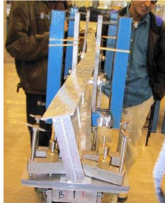
Lateral-torsional buckling of an aluminium alloy plate girder designed and built by students at Imperial College London.
