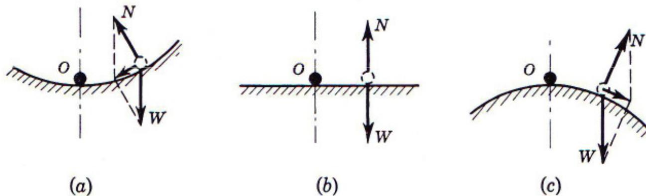
Fig. 9.1 Example of (a) stable, (b) neutral, and (c) unstable equilibrium.
