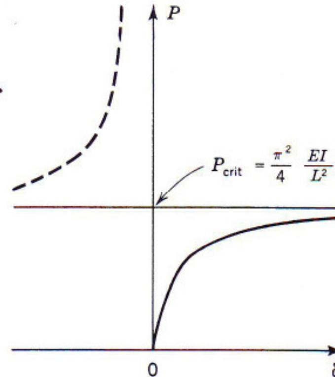
Fig. 9.14 Relation between compressive force  $P$  and transverse deflection  $\delta$  due to eccentricity  $\varepsilon$ .
