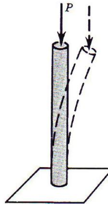
Fig. 9.7 Buckling of a column under a compressive load.
