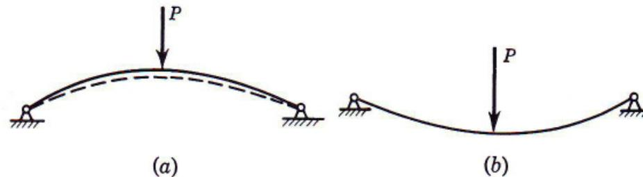
Fig. 9.10 “Snap-through” instability of a shallow curved member.
