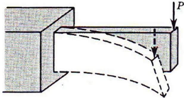
Fig. 9.6 Twist-bend buckling of a deep, narrow beam.
