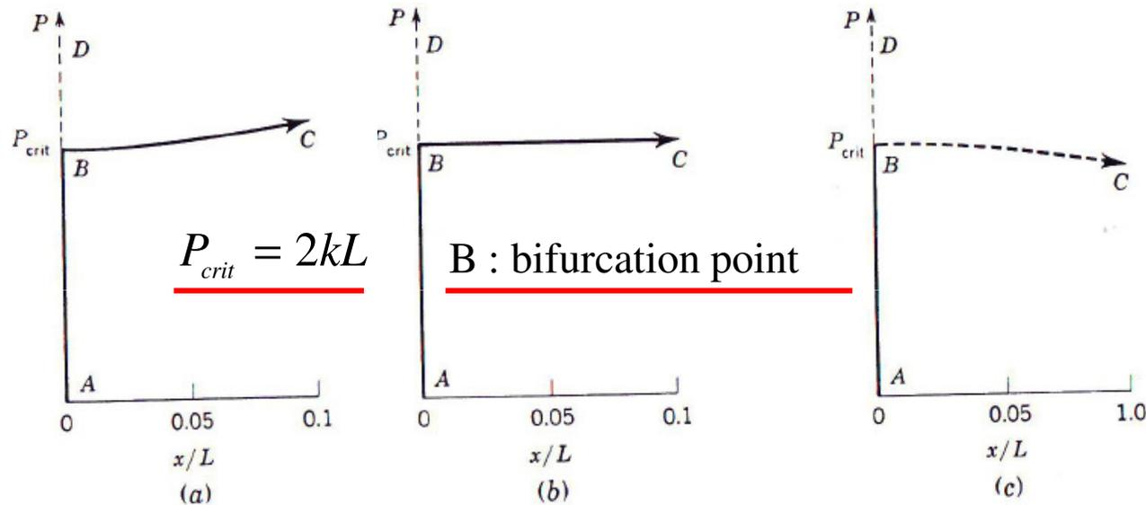
Fig. 9.17 Ideal postbuckling curves for (a)  $\beta = 10$ , (b)  $\beta = 0$ , (c)  $\beta = -10$ .
