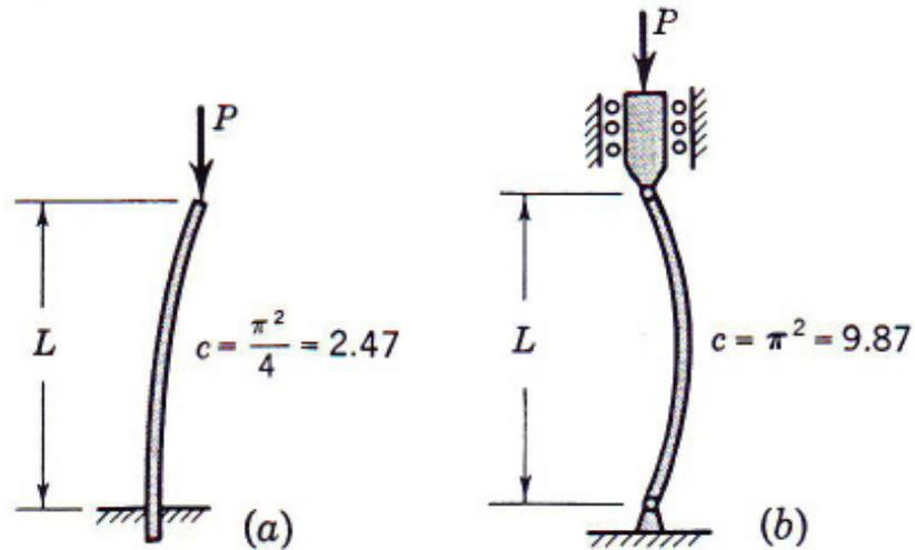
Fig. 9.15 Critical loads for (a) clamped-free, (b) hinged-hinged, (c) clamped-hinged, and (d) clamped-clamped columns. In each case the constant  $c$  shown is to be inserted in the formula  $P_{\text{crit}} = cEI/L^2$ .
