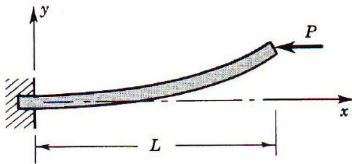
Fig. 9.12 Column in a state of neutral equilibrium in the bent position.
