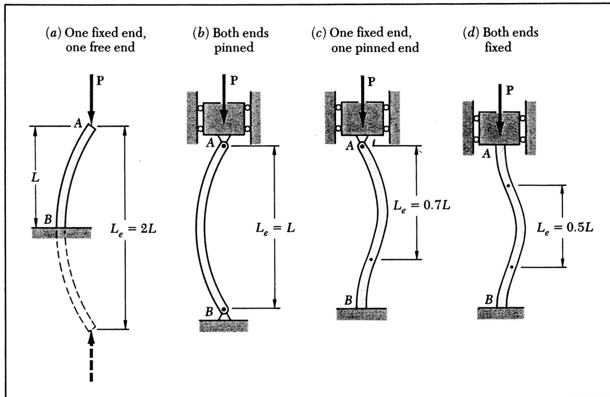
Fig. 11.17 Effective length of column for various end conditions.
