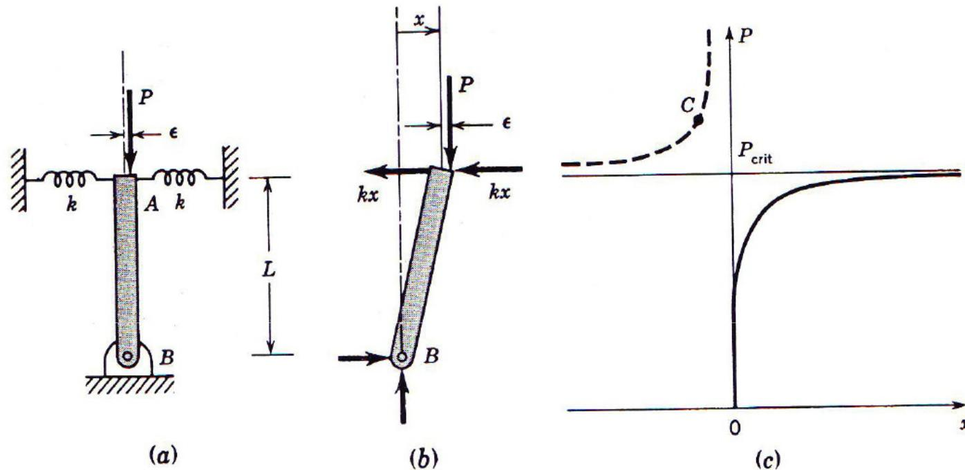
Fig. 9.4 Transverse displacement  $x$  due to load eccentricity  $\mathcal{E}$ .
