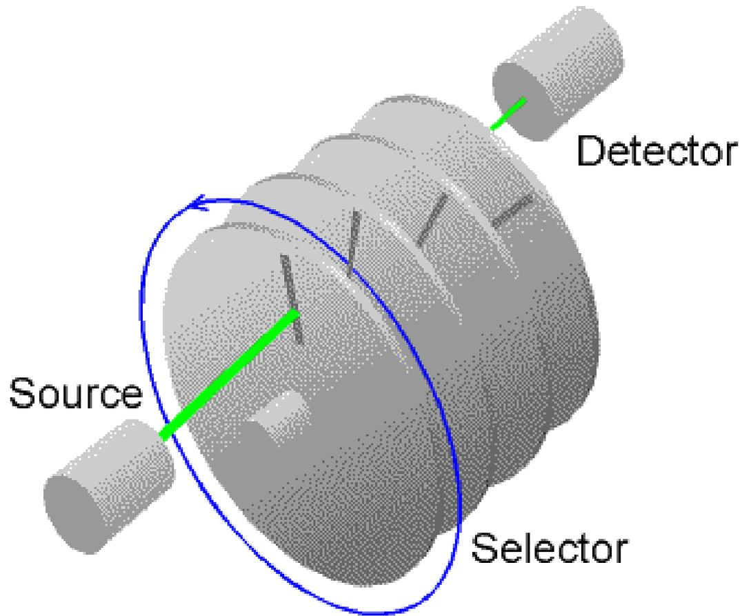
**Figure 20.9** A velocity selector. The molecules are produced in the source (which may be an oven with a small hole in one wall), and travel in a beam towards the rotating disks. Only if the speed of a molecule is such as to carry it through each slot that rotates into its path will it reach the detector. Thus, the number of slow molecules can be counted by rotating the disks slowly, and the number of fast molecules counted by rotating the disks rapidly.
