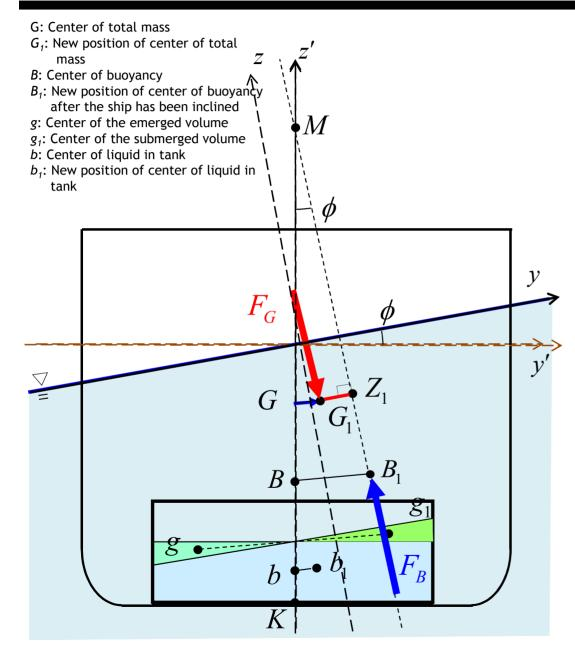
• When the ship is inclined, the liquid in the tank is also inclined. And the center of mass of the liquid shifts toward the inclined side.
