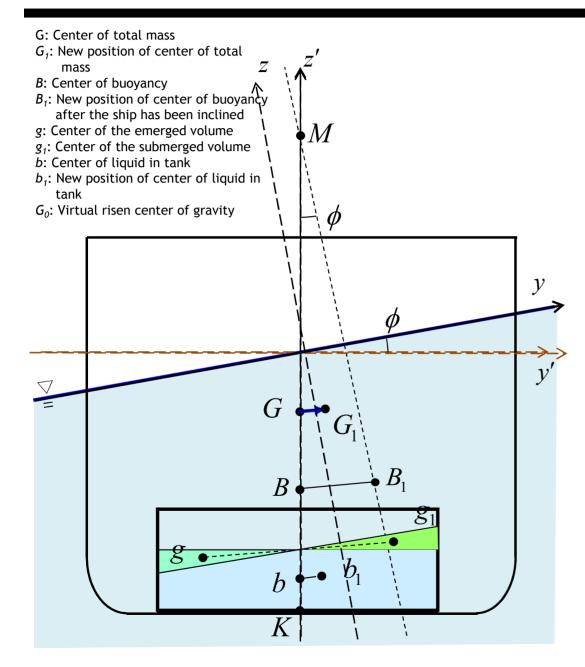
$\checkmark$  The effects of free surface depend on the dimensions of the surface of the liquid.
