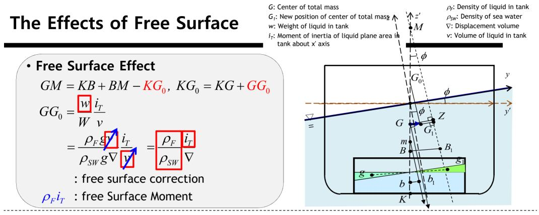
• The effects of free surface do not depend on the amount of liquid in the tanks.
