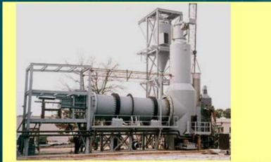
Rotary Kiln Waste Incinerator Plant with Vertical Thermo-Reactor
