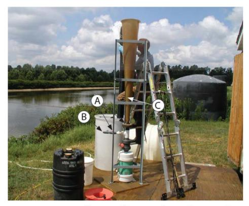
gure 1. Stuvite crystallizer used for 1.4 gal/min. flow rate of vered digester liquid. A) Add chemicals for Mg and pH inease at bottom of crystalizer cone or in inflow line; B) Wasteater inflow; C) Struvite crystals in bottom of cone
