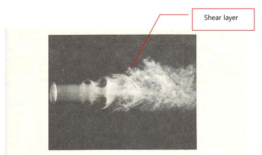
*Figure 9.2* Flow visualization of a turbulent jet at a Reynolds number of  $10.5 \times 10^4$ . [Courtesy of Steven Crow and Cambridge University Press.]
