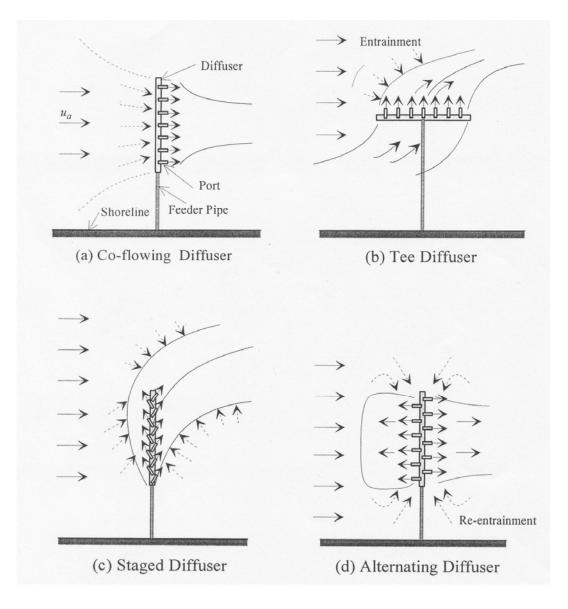
Types of submerged multiport diffuser
