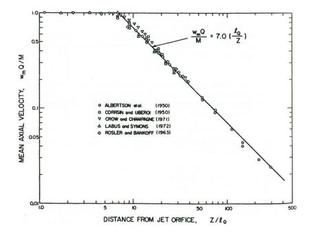
Fig. 2.5 Decay of peak time-averaged velocity on the axis of a round turbulent jet
