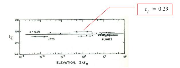
• Mean dilution in turbulent buoyant plane jets and plumes
