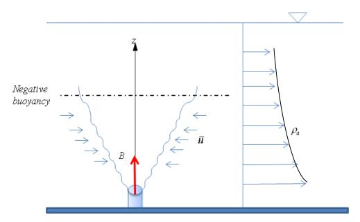
When a turbulent buoyant jet is rising in a density-stratified environment, the fluid entrained
