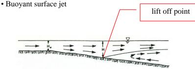
~ is likely to remain attached to the bottom for some distance, and then to spring from the bottom because of buoyancy.
