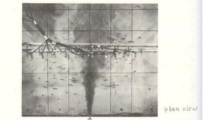
*Figure 9.31* A horizontal buoyant jet discharging into a laboratory flume. In the range shown the jet is attached to the bottom and momentum effects are dominant. [Photograph by B. Safaie.]
