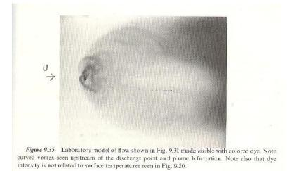
2) Horizontal buoyant jet into a crossflow  $\rightarrow$  Fig. 2.36
