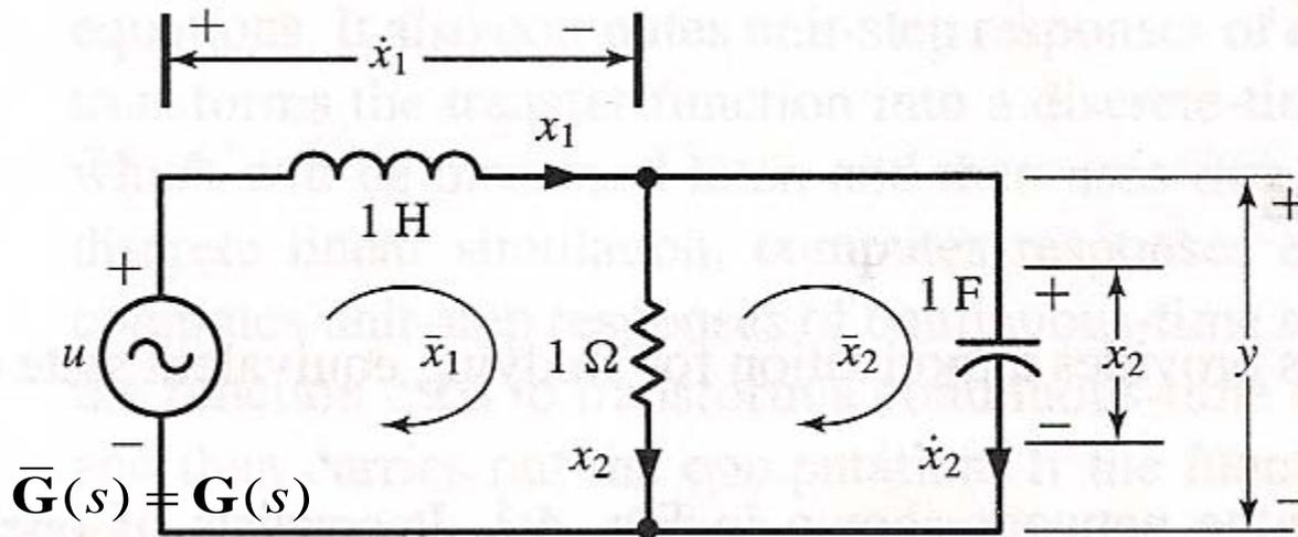
state1: Inductor current  $x_1(t)$ , Capacitor voltage  $x_2(t)$
