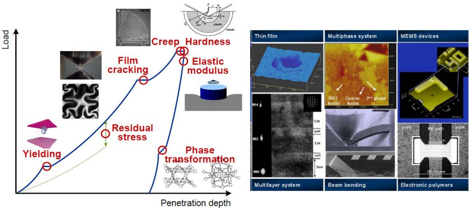
Accurate measurement at nano-scale without specific sample preparations
