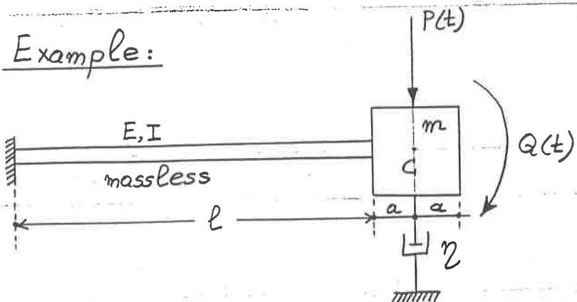
Consider a massless cantilever beam supporting a heavy rigid block.
