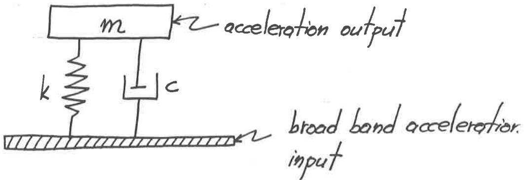
The base of the model is undergoing a broad band acceleration.
