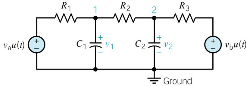
$$\text{node 1: } C_1 \frac{dv_1}{dt} + \frac{v_1 - v_a}{R_1} + \frac{v_1 - v_2}{R_2} = 0$$
