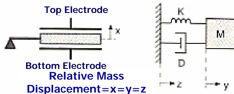
General accelerometer structure and its mechanical lumped model.
