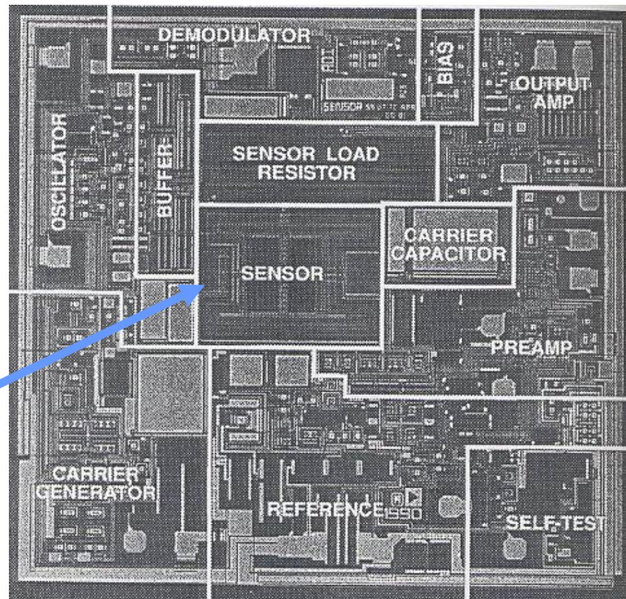
ADXL 50 accelerometer. The sensing element in the center is surrounded by active electronics. Chip size is 3 mm x 3 mm.
