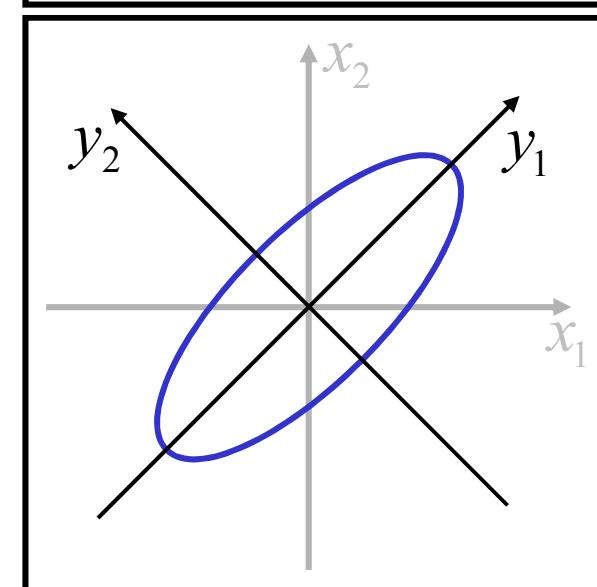
→ This means a 45° rotation (of principal axes. (See example 8.2-1.)
