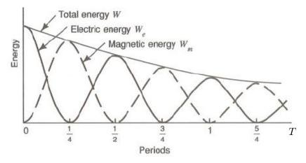
Quality factor Q: a measure of the bandwidth of a resonator
