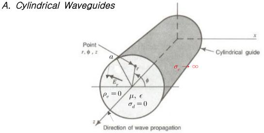
1) TE wave fields in the cylindrical waveguide
