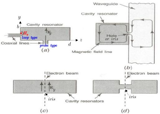
(e.g.)  $TE_{101}$  mode in an  $a \times b \times d$  rectangular cavity :
