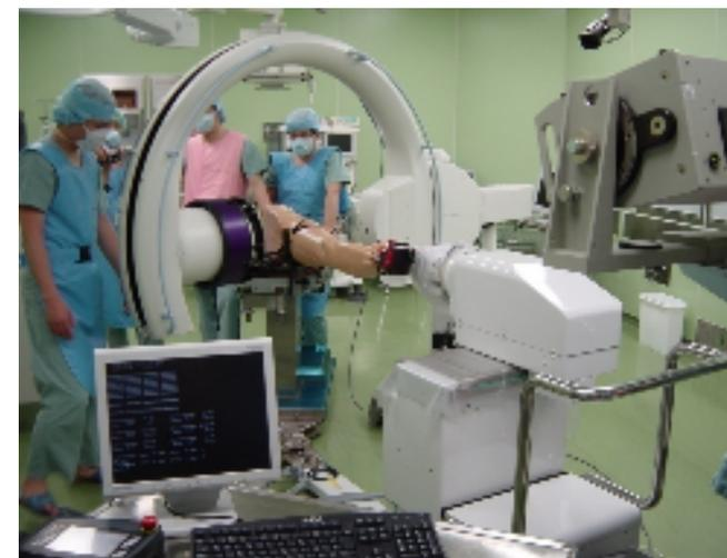
▲ Robot to assist femur fracture reduction
