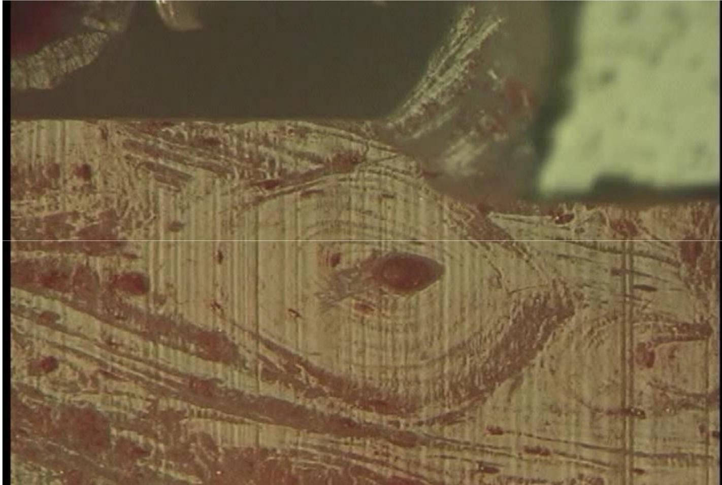
Cow, cortical bone, wet, depth of cut: 80 micrometer
