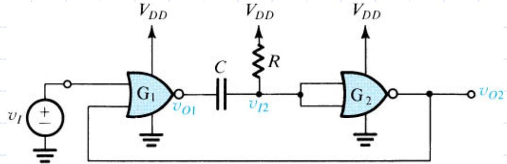
To generate an output pulse of duration  $T=1s$ ,  $R=?$
