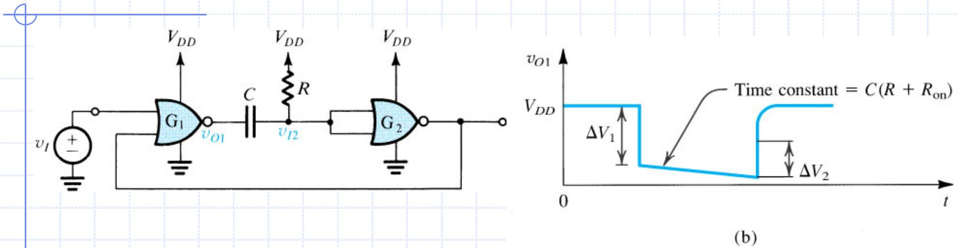
2. Trigger pulse is applied: The output of  $G_1$  will go low (but its output will not go all the way to 0V). The output of  $G_1$  drops by a value  $\Delta V_1$ .
