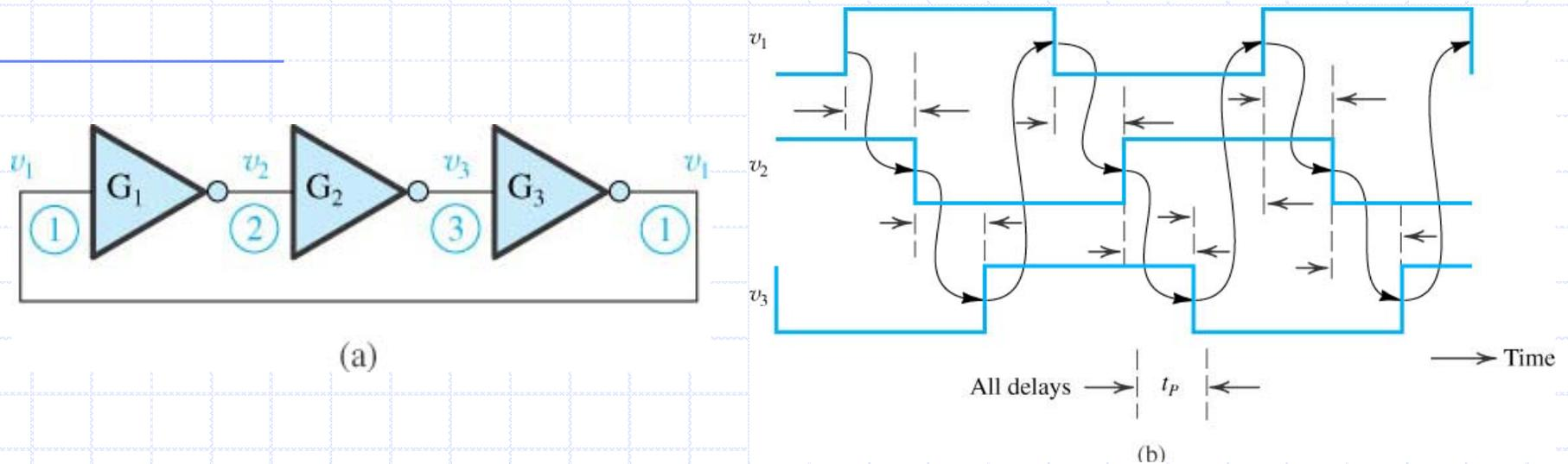
**Figure 11.16** (a) A ring oscillator formed by connecting three inverters in cascade. (Normally at least five inverters are used.)
