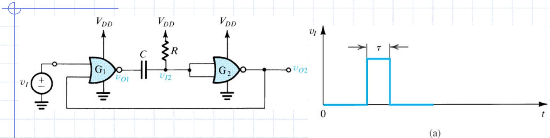
1. Stable state of the monostable circuit (the state of the circuit before the trigger pulse is applied): The output of  $G_1$  is high at  $V_{DD}$ , the capacitor is discharged, and the input voltage to  $G_2$  is high at  $V_{DD}$ .
