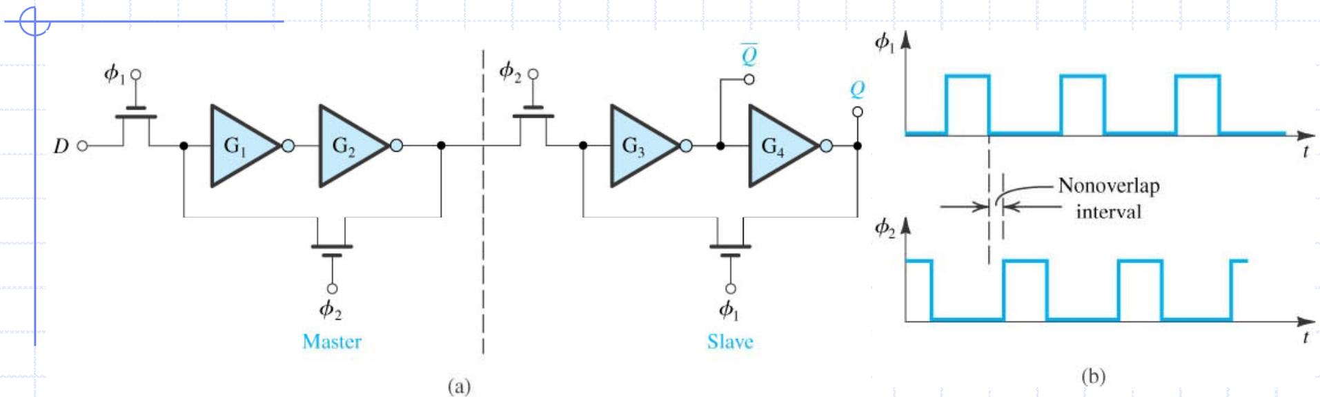
**Figure 11.8** (a) A master–slave D flip-flop. The switches can be, and usually are, implemented with CMOS transmission gates. (b) Waveforms of the two-phase nonoverlapping clock required.
