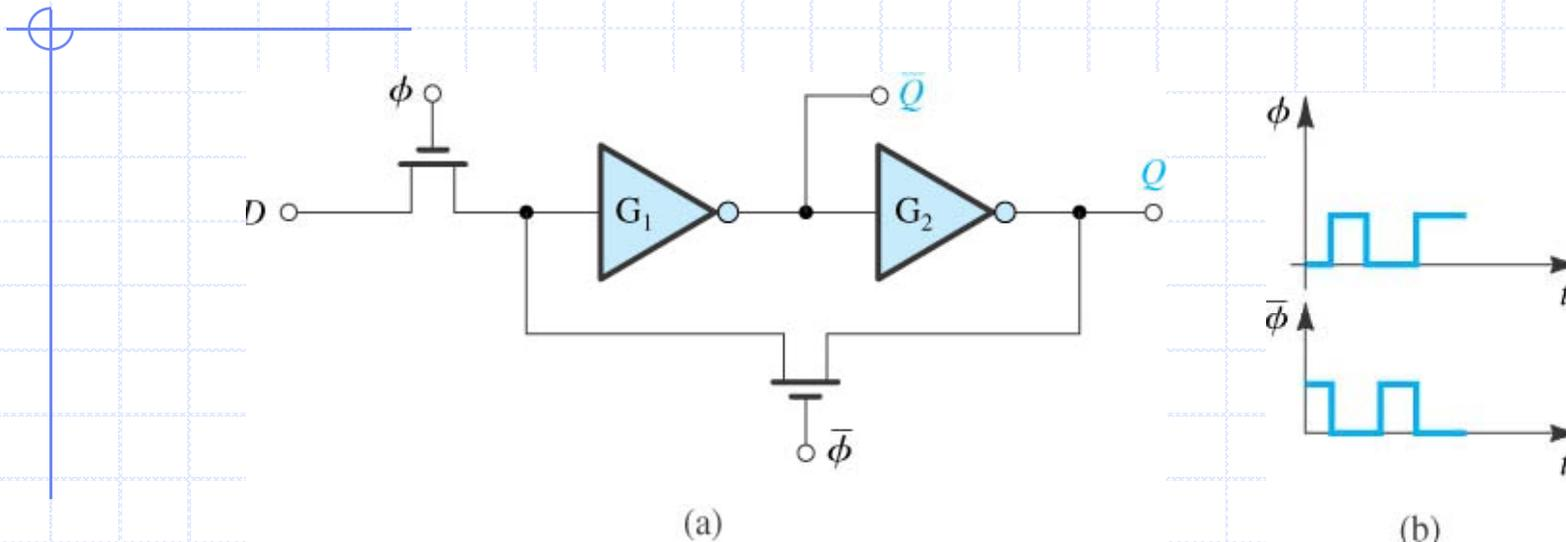
Figure 11.7 A simple implementation of the D flip-flop.
