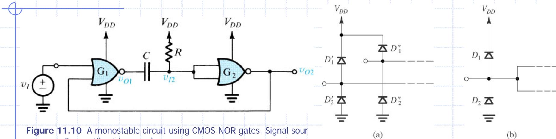
**Figure 11.10** A monostable circuit using CMOS NOR gates. Signal source  $v_I$  supplies positive trigger pulses.
