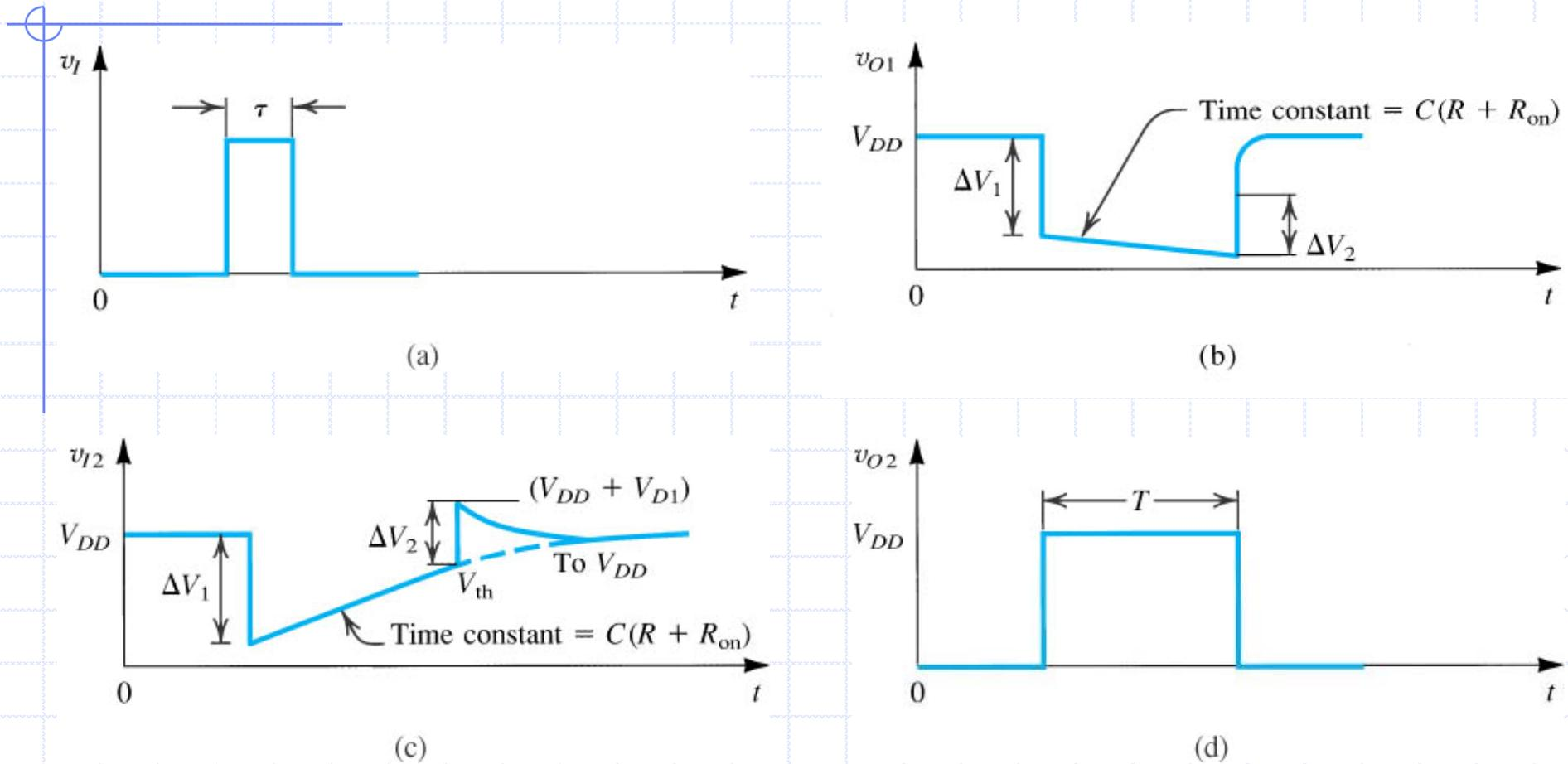
Figure 11.13 Timing diagram for the monostable circuit in Fig. 11.10.
