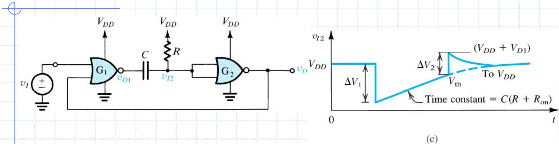
3. Operation in the quasi-stable state : The current through  $R$ ,  $C$ , and  $R_{on}$  causes  $C$  to charge, and the voltage  $V_{I2}$  rises exponentially toward  $V_{DD}$  with a time constant  $C(R + R_{on})$ .
