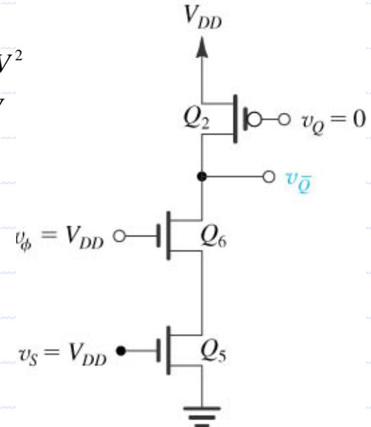
The four NMOS transistors in the set-reset circuit have equal  $W/L$  ratios. Determine the minimum value required for this ratio to ensure that the flip-flop will switch.
