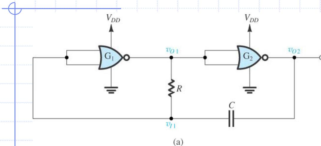
**Figure 11.15** (a) A simple astable multivibrator circuit using CMOS gates. (b) Waveforms for the astable circuit in (a). The diodes at the gate input are assumed to be ideal and thus to limit the voltage  $v_{i1}$  to 0 and  $V_{DD}$ .
