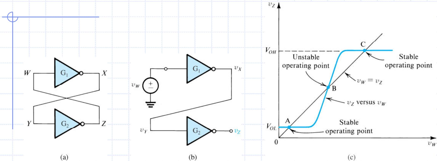
Figure 11.1 (a) Basic latch. (b) The latch with the feedback loop opened. (c) Determining the operating point(s) of the latch.
