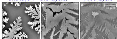
Evolution of the dendritic shape of pentacene islands on cyclohexene-saturated Si(001).
