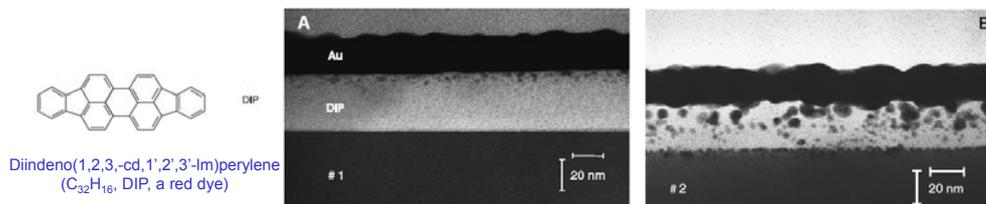
Fig. 8 Cross-sectional TEM images of two Au/DIP/siliconoxide heterostructures. While the Au contact prepared at  $-120^{\circ}\text{C}$  and a rate of  $23 \text{ \AA}/\text{min}$  (left) exhibits rather well-defined interfaces, the Au contact prepared at  $70^{\circ}\text{C}$  and a rate of  $0.35 \text{ \AA}/\text{min}$  (right) shows strong interdiffusion. Note that individual lattice planes of the DIP film can be resolved. From Ref. [50] with permission.
