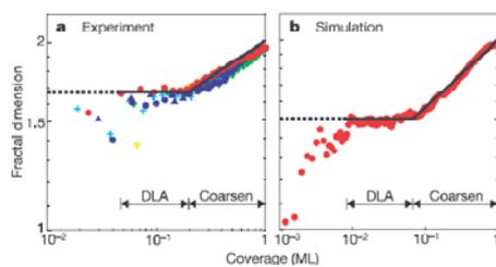
Figure 4 Coverage-dependent fractal dimension of single-molecular-layer pentacene islands on cyclohexene-saturated Si(001). **a**, Experiment; **b**, modified DLA (diffusion-limited aggregation) simulation. Independently of the experimental conditions, including growth rate variations and substrate surface preparation as illustrated by the different colours and symbols, the fractal dimension follows a universal curve.
