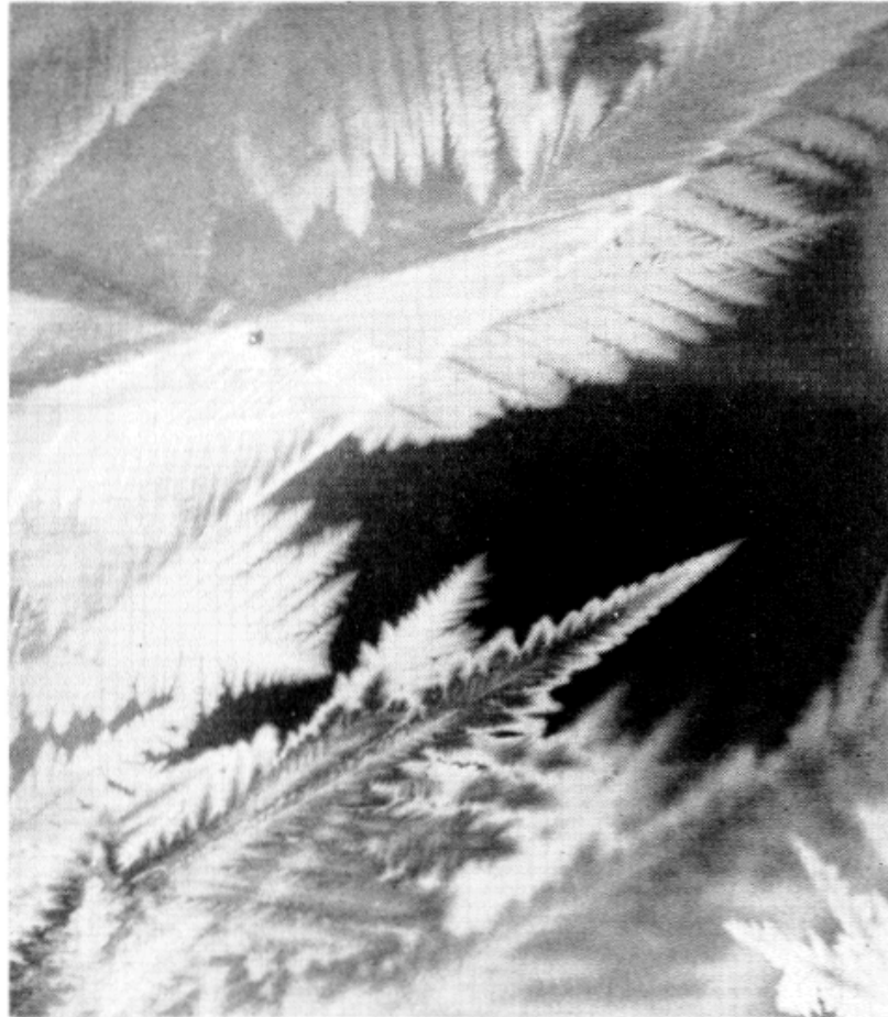
Fig. 4.12. Dendritic morphology of ice growing in water at -1.5^{\circ}\text{C} . Photograph by R. B. Williamson.
