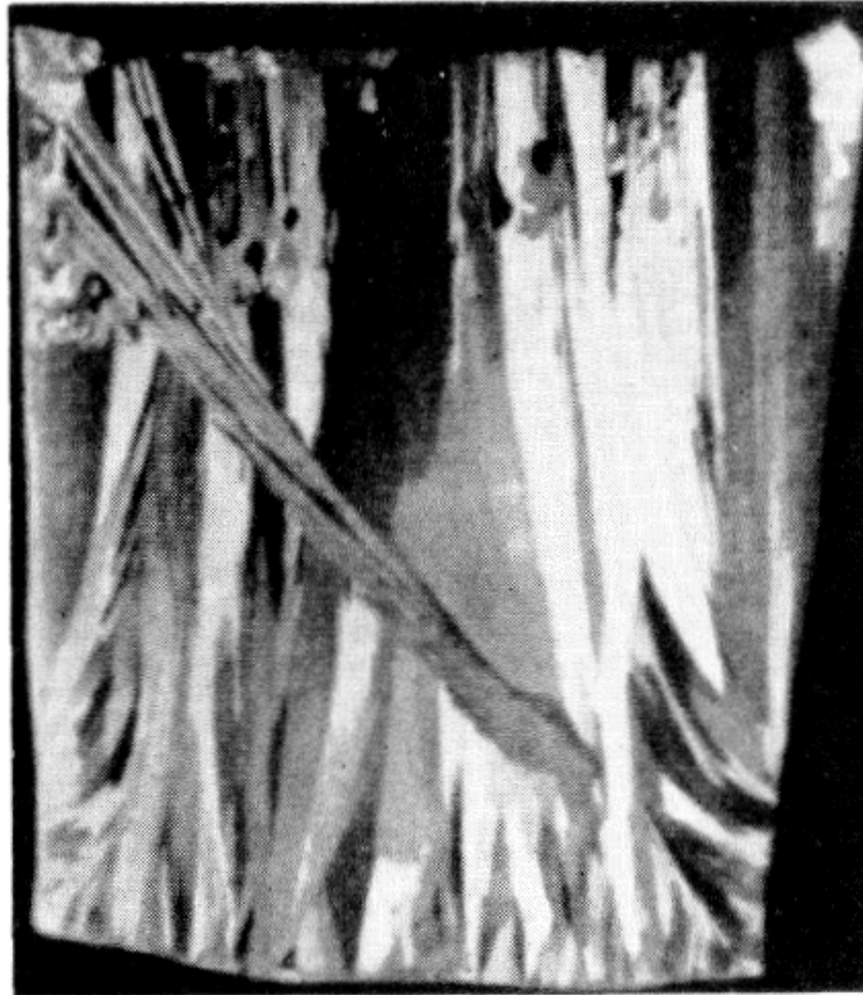
Fig. 4.11. “Feather” crystals. [From Brenner and Roth, Z. Metallkunde , 32 , 10 (1940).]
