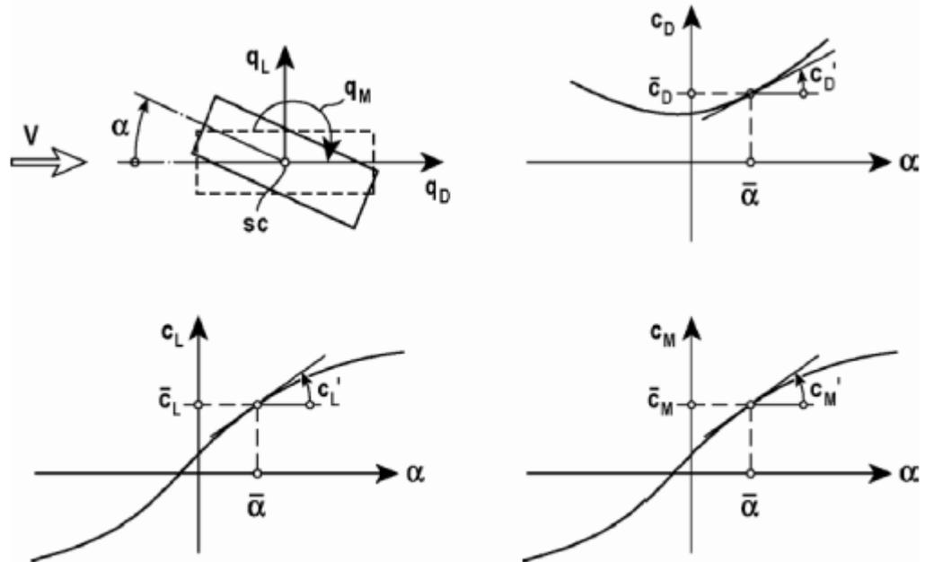
Fig. 5.2 Load coefficients obtained from static tests
