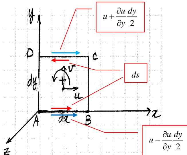
– take line integral from A to B, C, D, A ~ infinitesimal CV
