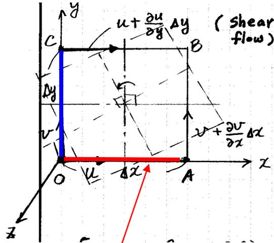
Assume the rate of rotation of fluid element  $\Delta x$  and  $\Delta y$  about  $z$ -axis is positive when it rotates counterclockwise.
