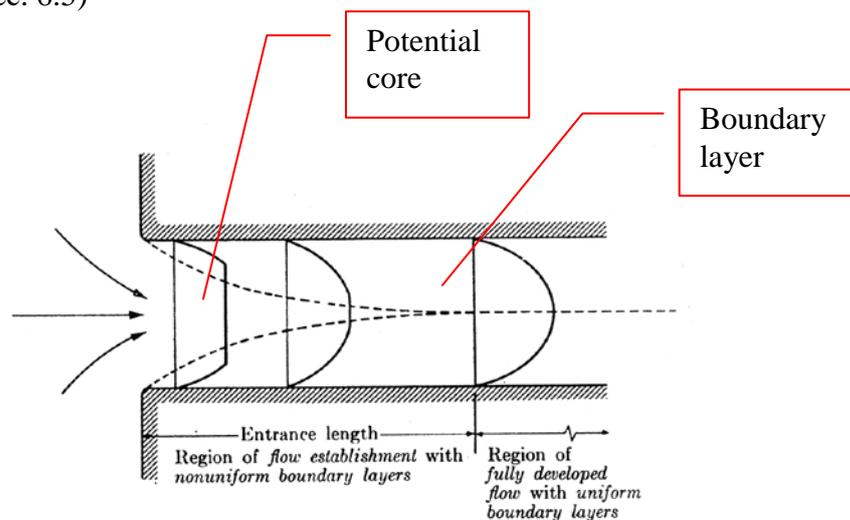
FIG. 8-5. Boundary layers in ducts.
