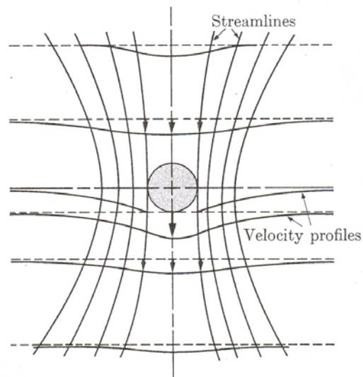
FIG. 8-3. Deformation flow around a falling sphere. (Streamlines and velocity profiles are shown for observer at rest.)
