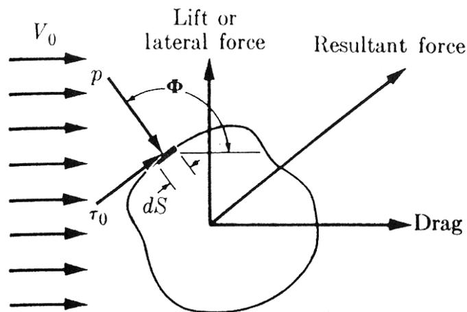
FIG. 8-7. Definition diagram for flow-induced forces.
