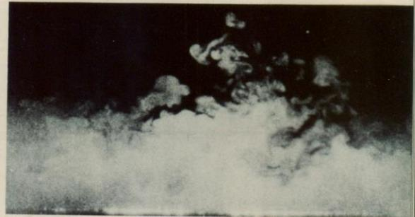
163. Oblique transverse sections of a turbulent boundary layer. The flow is viewed head-on, with smoke illuminated by a sheet of light that is inclined  $45^\circ$  downstream from the wall on the left and  $45^\circ$  upstream on the right.
