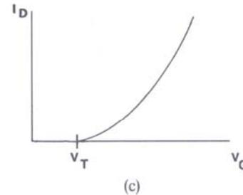
Figure 8.29. (a) Enhancement (normally-off)-type  $n$ -channel MOSFET. For details, see the caption of Fig. 8.28. (b) Circuit symbol. (The broken line indicates that the path between S and D is normally interrupted.) (c) Gate voltage ( $V_G$ )/drain current ( $I_D$ ) characteristic.  $V_T$  is the threshold gate voltage above which a drain current sets in.
