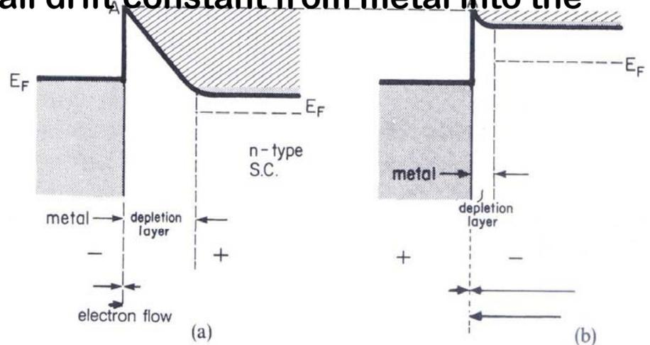
Figure 8.15. Metal–semiconductor contact with two polarities: (a) reverse bias and (b) forward bias. The number of electrons that flow in both directions and the net current is indicated by the length of the arrows. The potential barriers are marked by heavy lines.
