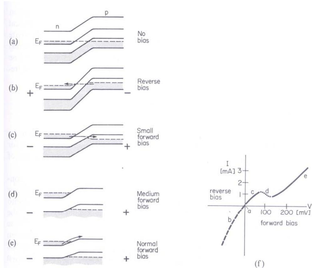
Figure 8.24. (a)–(e) Schematic energy band diagrams for highly doped  $n$ - and  $p$ -type semiconductors (tunnel diode). (a) No bias. (b) Reverse bias. (c) Small forward bias. (d) Medium forward bias. (e) “Normal” forward bias. (f) Voltage–current characteristic for a tunnel diode.
