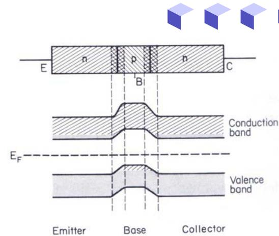
Figure 8.25. Schematic band diagram of an unbiased *n-p-n* bipolar junction transistor.
