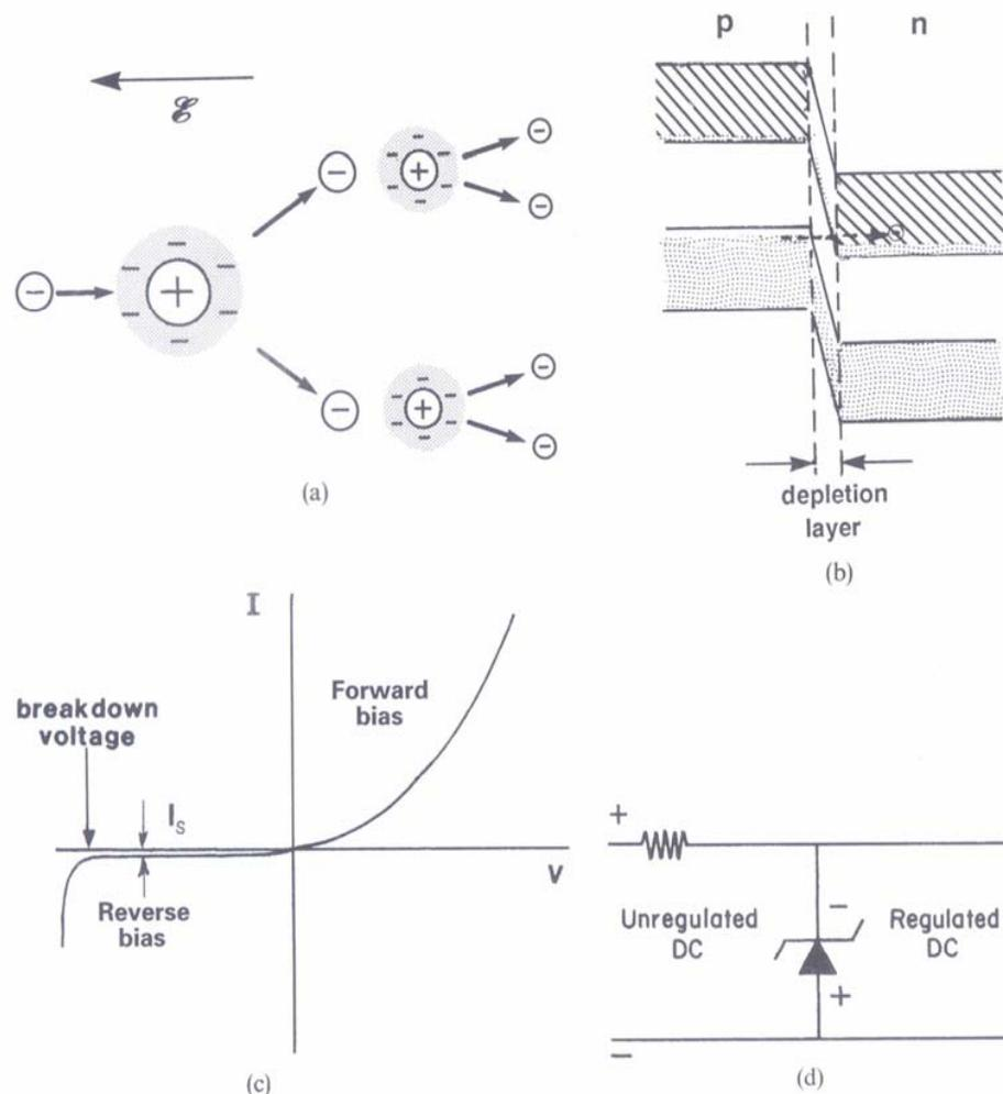
Figure 8.20. (a) Electron avalanche created at breakdown voltage. (b) Tunneling (Zener breakdown). (c) Voltage-current characteristic of a p-n diode exhibiting a breakdown voltage at a large reverse voltage. As in Fig. 8.16(a),  $I_s$  is shown grossly exaggerated. (d) Zener diode in a circuit for voltage regulation.
