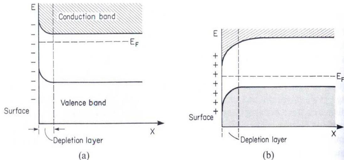
Figure 8.12. (a) Band diagram for an *n*-type semiconductor whose surface has been negatively charged. (b) Band diagram for a *p*-type semiconductor, the surface of which is positively charged. *X* is the distance from the surface.
