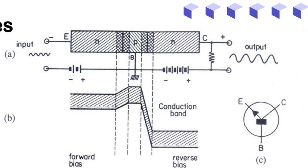
Figure 8.26. (a) Biasing of an  $n-p-n$  bipolar transistor. (b) Schematic band diagram (partial) of a biased  $n-p-n$  bipolar transistor. (c) Symbol used for a bipolar  $n-p-n$  transistor.
