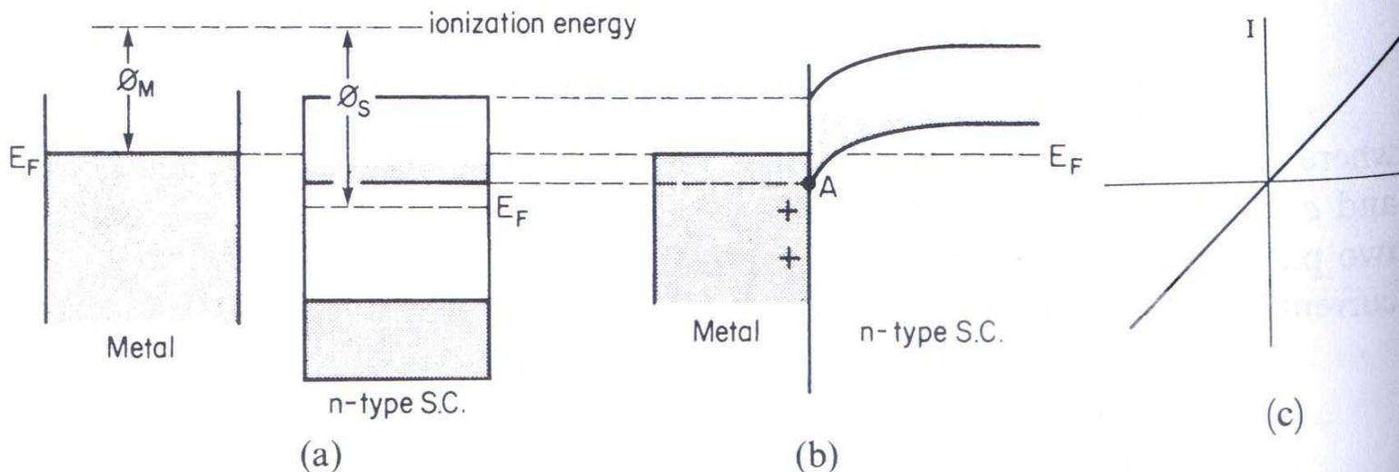
Figure 8.17. Ohmic contact between metal and *n*-type semiconductor ( $\phi_M < \phi_S$ ). (a) Metal and semiconductor are separate. (b) Metal and semiconductor are in contact. (c) Current-voltage characteristic.
