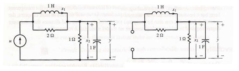
When u = 0,  $x_1(0) = a \neq 0$ ,  $x_2(0) = 0$ , the output y(t) = 0. There is no way to determine the initial state [a, 0]form y(t) and u(t).  $\Rightarrow$  unobservable
