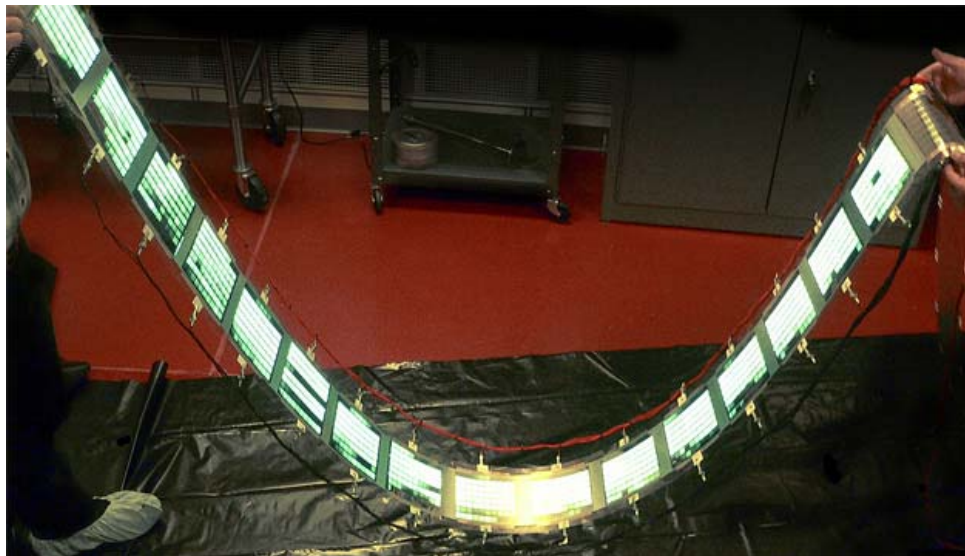
8-ft. strip comprised of 6 x 6 in. lighting panels GE / Energy Conversion Devices / NIST the 2008. 3.
