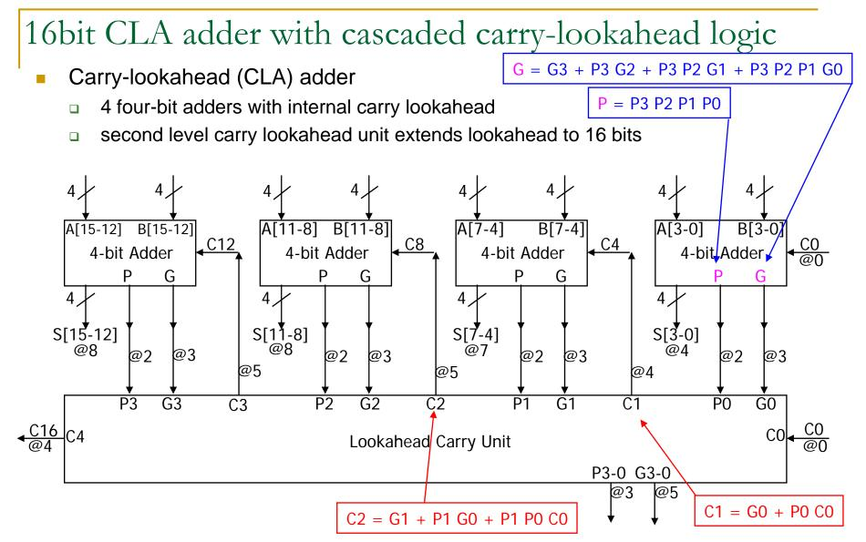
If we add 16bit long numbers, we have to use 4 4bit CLA adder modules. Each module adds 4 bits. Here Ci at the bottom box is the carry from the i-th 4bit CLA adder module. Pi and Gi in blue color are the same functions in the previous example. While Pi and Gi at the bottom unit give info about the carries between the 4bit CLA modules, which is more complicated.
