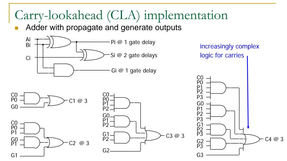
This slide shows how 4 carries are implemented in two level fixed logic based on Pi and Gi. As Pi and Gi take only one gate delay, the final carries take maximum 3 gate delays.
