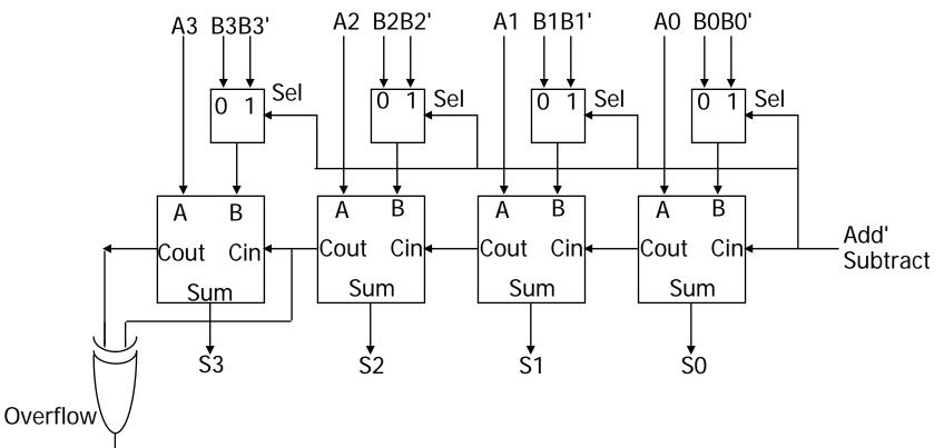
Now we have a full adder for one bit addition. Then what we want to do is addition/subtraction of two 4bit-numbers. Addition is easy. Recall that 2s complement of a number is its inverted form+1. So we can use the same adding function to perform subtraction too. For subtraction, we just enable the control input.
