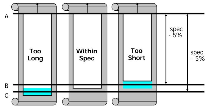
What if we don't have sensor A? We cannot know the reference point or time at which we can measure the length of each rod. So when sensor A becomes 1, we should check sensors B and C as well to measure the length of the moving rod.
