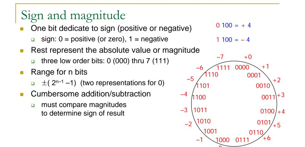
The first encoding scheme is sign and magnitude; one bit is dedicated to the sign of the number and the rest of the bits represents the absolute value of the number |x|. If we use 4 bits total, the MSB is the sign + or -, and the other three bits represent the magnitude from 0 to 7. The problem is that when adding or subtracting numbers, we have to check the sign of the results.
