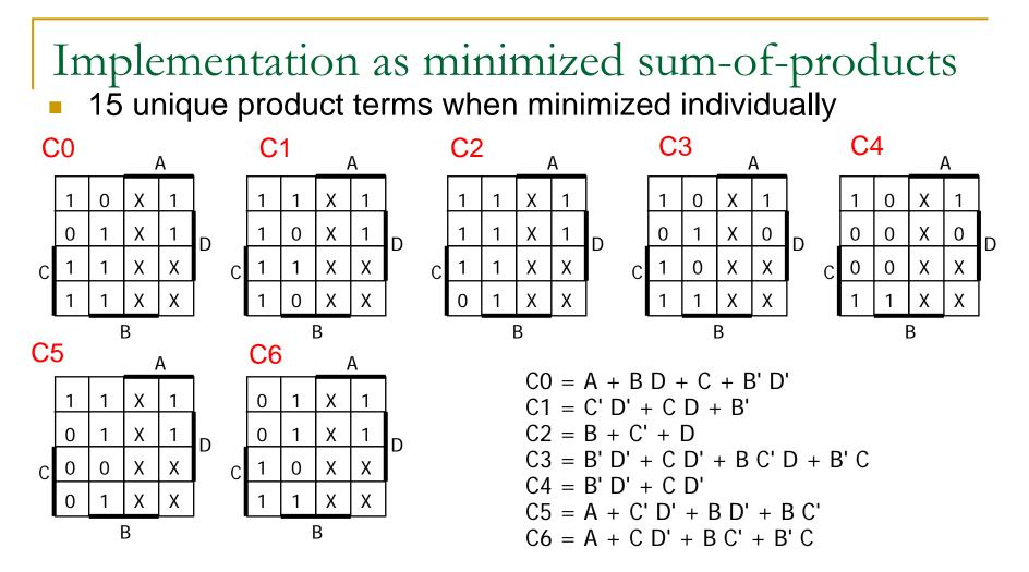
Here are the final two-level s-o-p forms for 7 output functions. After removing duplicate product terms, we have 15 different product terms to represent 7 outputs. We should note that the minimized form of each output may not lead to the globally minimum number of product terms. In this case, we have 15 product terms for 7 outputs
