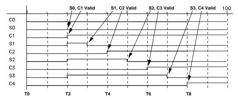
This slide shows a waveform of a 4 bit adder. Suppose we add 1111 and 0001, the carry will propagate from the LSB all the way through to the final carry-out.
