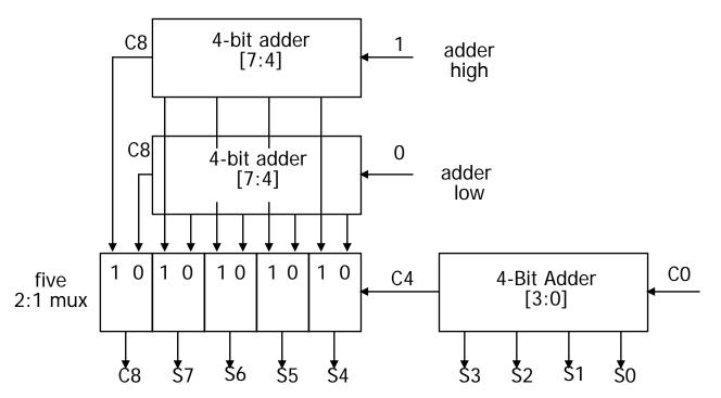
The next version, a carry-select adder, achieves even lower delay by redundant h/w. Note that the carry between 4bit CLA adders is either 0 or 1. We use two adder modules for high 4 bit of the 8-bit adder system. So we perform addition for both cases and then the carry from the lower 4bit CLA module will perform selection (MUX).
