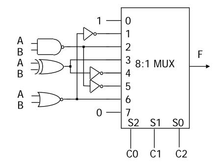
In order to realize the multi-purpose function, we combine discrete gates and an 8:1 MUX.
