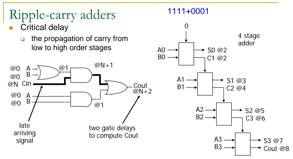
The next advanced adder is a ripple-carry adder. What is the problem of the full adder in the previous slide? When we consider data bits, they are coming in parallel at the same time. However, carries should be cascaded with delays proportional to the bit positions. On the left, Cin comes at time N, then Cout will be valid at time N+2 (each one-bit adder incurs 2 gate delays)
