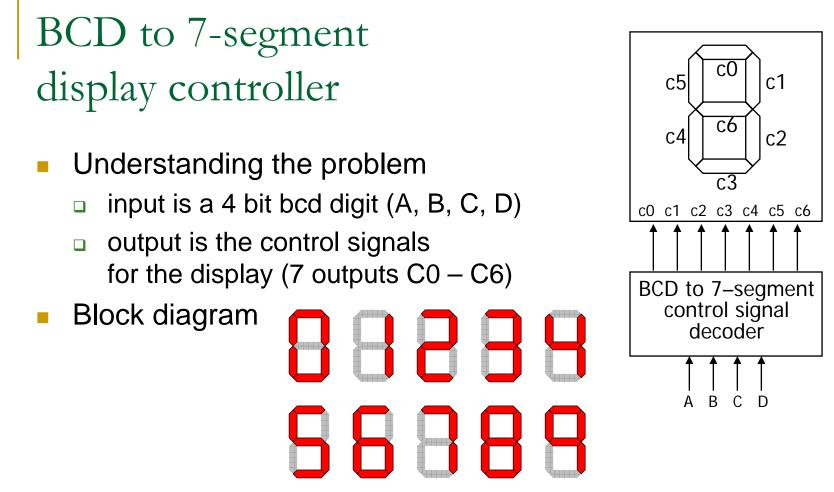
The first case is to control or display one digit system whose input follows BCD coding.
