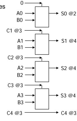
on the left, there is the original full adder, which takes a long time to finish addition. On the right, there is the carry lookahead adder. The two level logic functions for carries are not shown. Each box is the one-bit adder module. Overall, by using a lot of gates for CLA in the previous slide, we can reduce the delay of the addition process.
