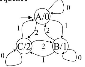
• Comparator: a FSM that receives two binary numbers and determine whether they are equal, lager, or smaller. We assume that the digits of the two numbers come in one by one, with the lower-order digits coming in first.
