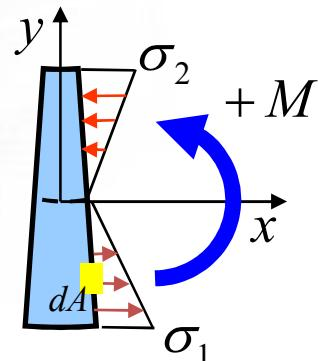
$$\begin{aligned}\therefore dM &= -y\sigma dA \\ &= -y dF\end{aligned}$$
