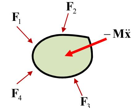
$$0 = \underline{F}_1 + \underline{F}_2 + \underline{F}_3 + \underline{F}_4 - \underline{M}\ddot{x}$$
