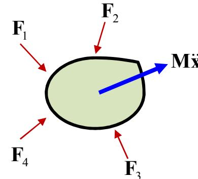
$$\underline{M}\ddot{x} = \underline{F}_1 + \underline{F}_2 + \underline{F}_3 + \underline{F}_4$$
