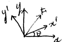
$$\underline{F} = F_x \underline{e}_x + F_y \underline{e}_y = F_{x'} \underline{e}_{x'} + F_{y'} \underline{e}_{y'}$$
