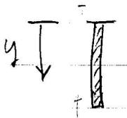
$$\cancel{\frac{\partial T_{yy}}{\partial x}} + \frac{\partial T_{yy}}{\partial y} + \cancel{\frac{\partial T_{xy}}{\partial z}} + F_y = 0$$
