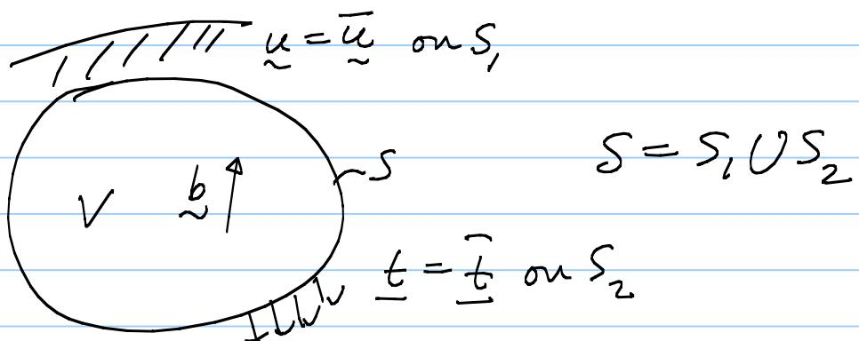
Assume two solutions  $(\underline{u}^{(1)}, \underline{\sigma}^{(1)})$  and  $(\underline{u}^{(2)}, \underline{\sigma}^{(2)})$  satisfy the same load/boundary conditions:
