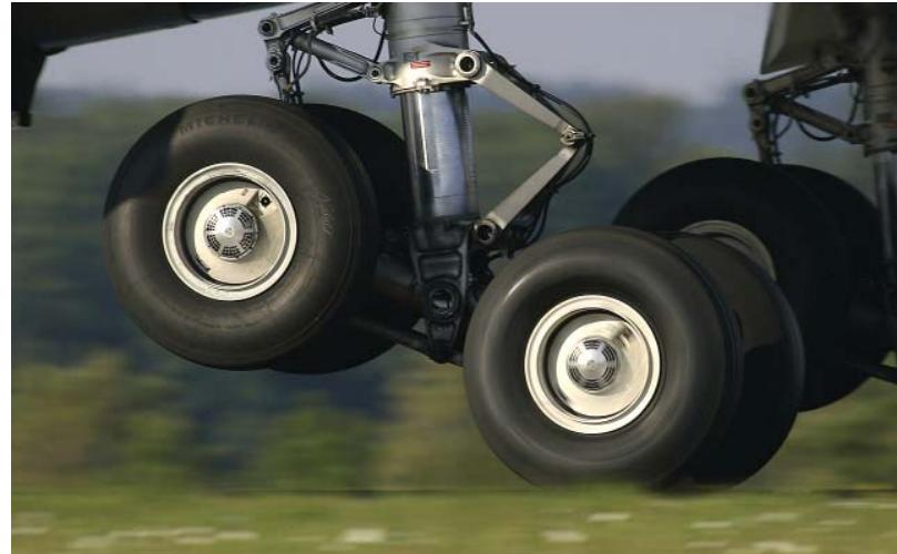
Landing gear system of AIRBUS A330
