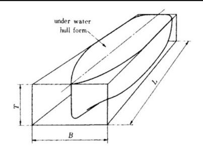
= Displacement / (L x B x T x Density) where, density of sea water = 1.025 [Mg/m<sup>3</sup>]
