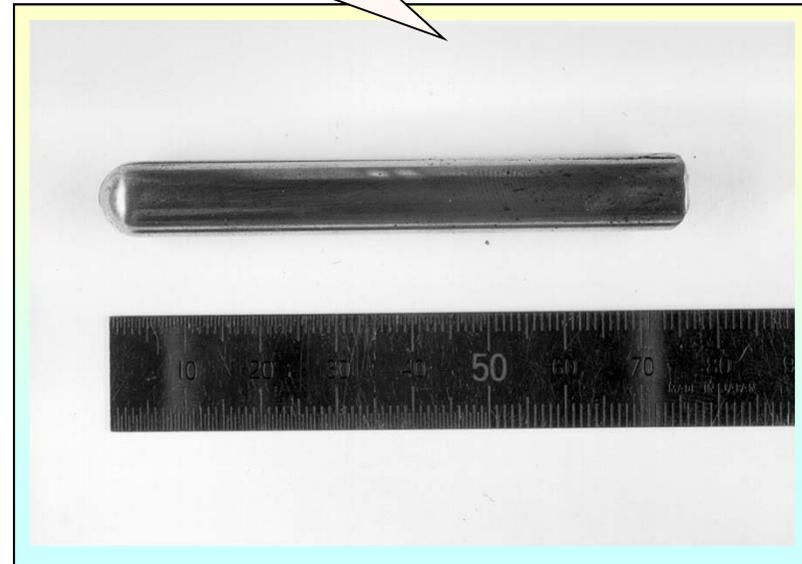
Push the molten alloy through hydraulic pressure into the Cu mold
