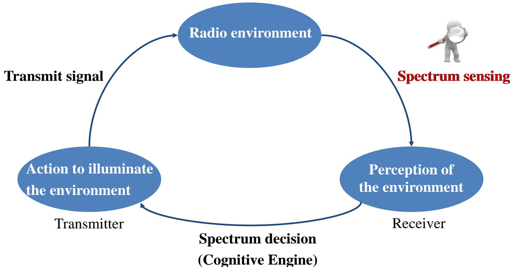
**Figure. Role of power spectrum sensing in cognitive radio networks**
