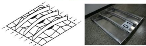
Mode III - stiffener-induced collapse by beam-column type collapse
