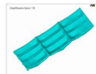
Figure 20(a) Three dimensional displays of a selected prototype structure distorted after welding (with amplification factor of 30), for ID 63
