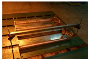
Figure 19(c) A photograph of initial distortion measurement for a stiffener in progress
