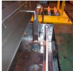
Figure 19(a) Dial gauge and its attachment for initial distortion measurement
