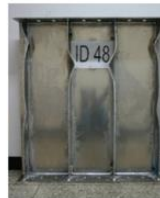
Mode V - stiffener-induced collapse by tripping
