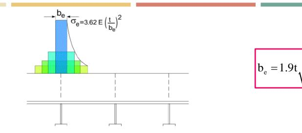
As the overall force on the deck increase and the effective width decreases, the von-Karman model will remain valid until the edge stress reaches yield. At this point, the frames will collapse. The minimum effective width can be found by substituting the yield stress into equation (7).
