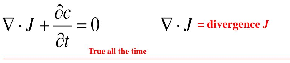
$$\therefore \frac{\partial c}{\partial t} = D \frac{\partial^2 c}{\partial x^2}$$
