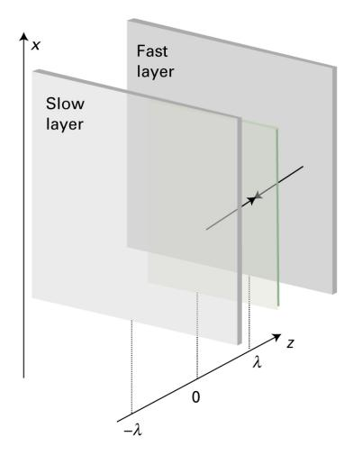
$$\eta = \frac{1}{3}m\lambda \widetilde{N}\overline{c} = \frac{1}{3}m\lambda \overline{c}N_A\left(\frac{n}{V}\right)$$
