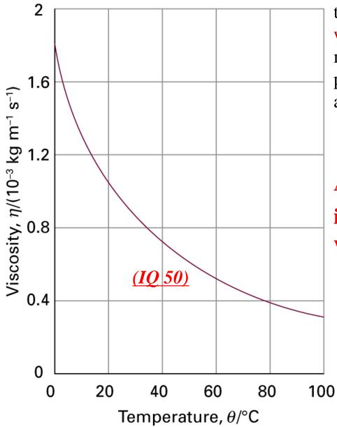
**Figure 19B.1.** The experimental temperature dependence of the viscosity of water. As the temperature is increased, more molecules are able to escape from the potential wells provided by their neighbors, and so the liquid becomes more fluid.
