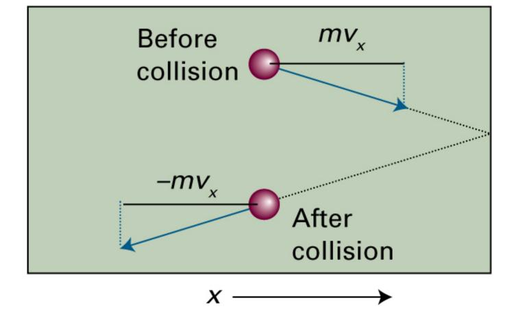
The pressure of a gas arises from the impact of its molecules on the walls. In **an elastic collision** of a molecule with a wall perpendicular to the *x*-axis, the *x*-component of velocity is reversed, but the *y*- and *z*-components are unchanged.
