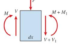
**Note:** No change in the bending moment, but dM/dx = V changes from V to  $V + V_1 = V - P$
